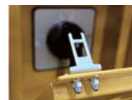
The panel of the voltage switch provides protection function, the engine will stop upon opening of the panel
