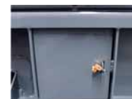
Drainage safety valve at the bottom of the fuel tank
