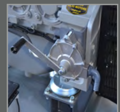
Oil change pump it facilitates oil change
