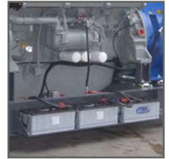
Battery holder designed to facilitate maintenance and replace
