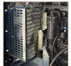
Heat and rotating part guards to prevent injuries to the user
